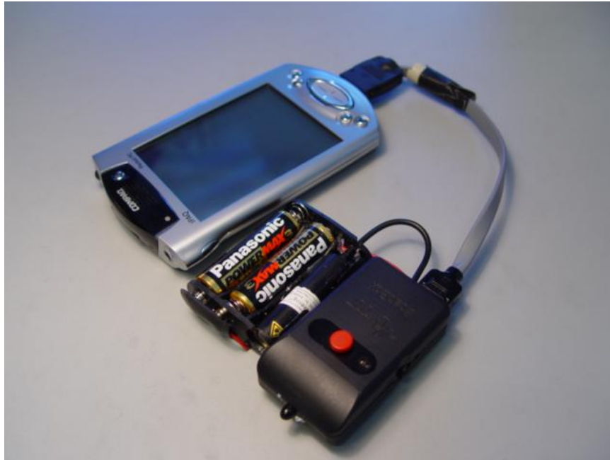
Fig. 2. The physical browser components: iPAQ (left), central SoapBox (right) and a laser beam unit (middle). The SoapBox has a pointing button (shown in the middle of the SoapBox) to activate the laser unit and the IR transmitter (visible in front of the SoapBox)
