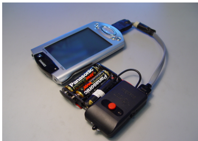
Figure 2. A physical browsing system. The iPAQ acts as a terminal device and the attached SoapBox module acts as a tag reader. The button on the SoapBox is used to trigger the pointing beam and the LED in front of the module sends an IR pulse to the remote tag. The battery case contains a laser pointer to aid in aiming.
