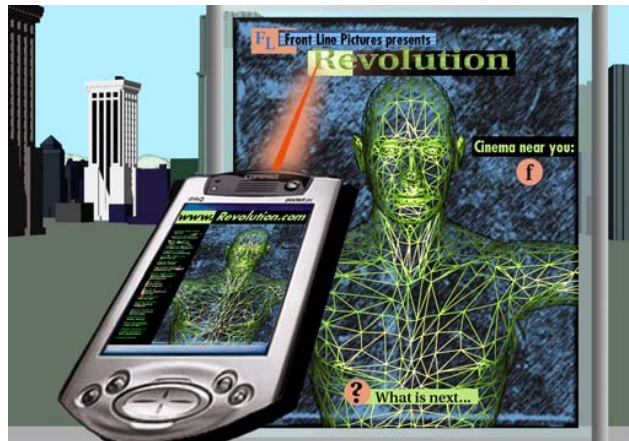
Figure 1. Physical browsing. The user points to a tag in a poster, and the mobile terminal loads a WWW page from the URL, which the tag provides.
