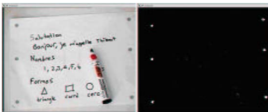
Fig. 1. Camera view looking at pen and paper (left), segmented green fiducials (right)
