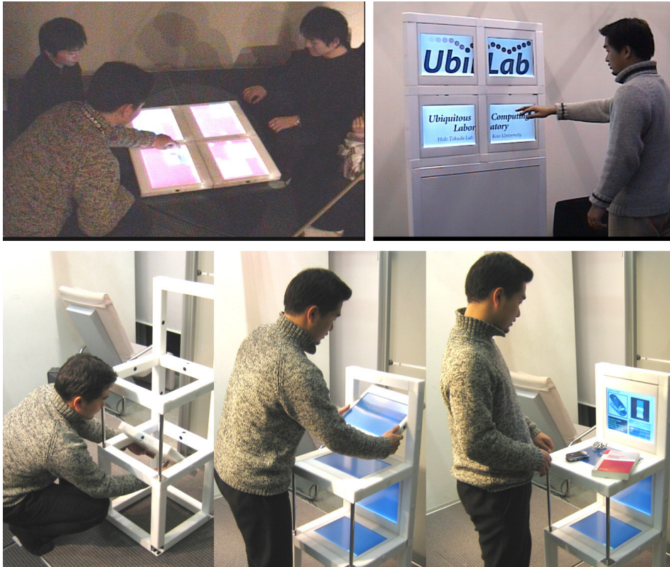
Figure 2. Smart Table (upper left), Smart Multi-display (upper right) and Smart Shelf (lower): u-Texture connects with other ones horizontally and vertically, and collaborates with each other by exchanging location and inclination information, commands, and data.
