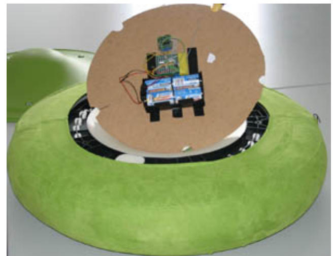
Figure 4: Opened Virrig with the integrated Smart-Its.
