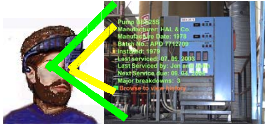
Figure 3. Head-mounted concept for Flashback device, with its foldable visor, projecting networked Logs of the equipment's history like hologram in the view of the worker; the projected image can also be pictures or video footages of past repair activities by the experienced for situated, peripheral learning at the scene of the task a novice worker
