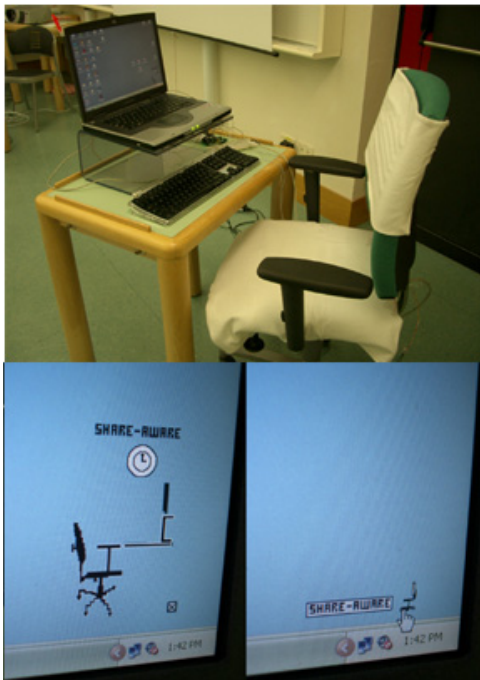
Figure 4: Shows the various components of our system that helps the user evaluate his workstation habits.
