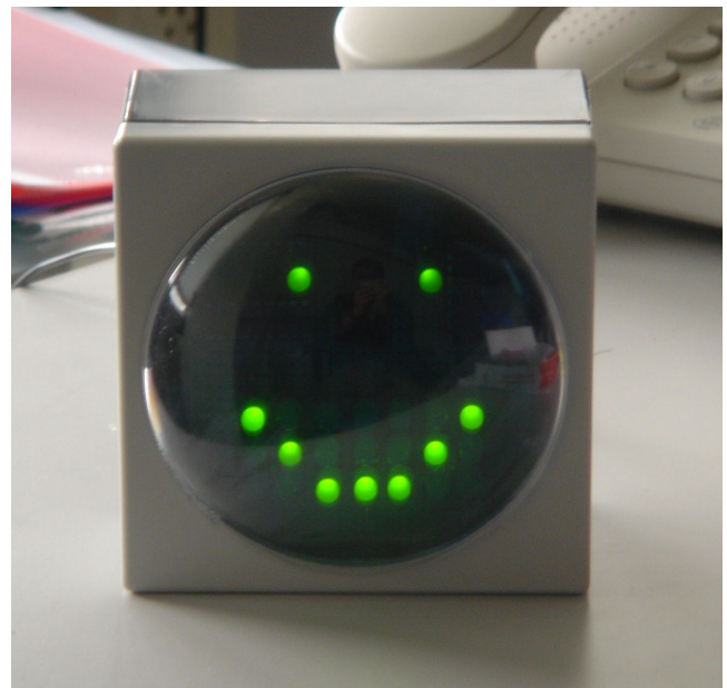
Figure 2 mPacer can detect the presence of a user and provide emotional expressions at the different stages during work.
