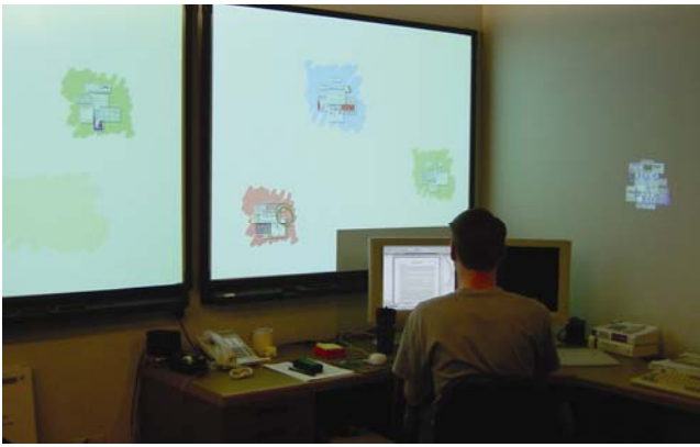
Figure 1. The Kimura system, including a desktop component, two interactive peripheral displays with electronic whiteboard capabilities, and a third non-interactive peripheral display. The images projected on the electronic whiteboards are montages , representations of activity that integrate history and context information.
