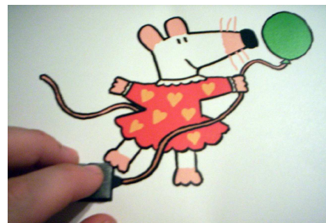
Figure 8. Interaction through a pressure sensor: the ball prototype
